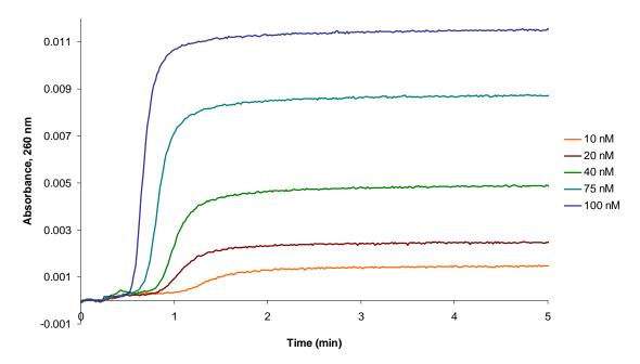
column (see figure below). Based on the time required for this breakthrough curve to appear when various concentrations of substrate are applied, a binding constant for the enzyme-substrate interaction can be determined. This project is in collaboration with Dr. Frank Kovacs.
